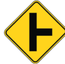
Side road enters highway ahead.
